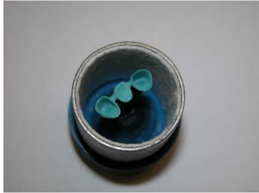
(28) Lined casting ring
