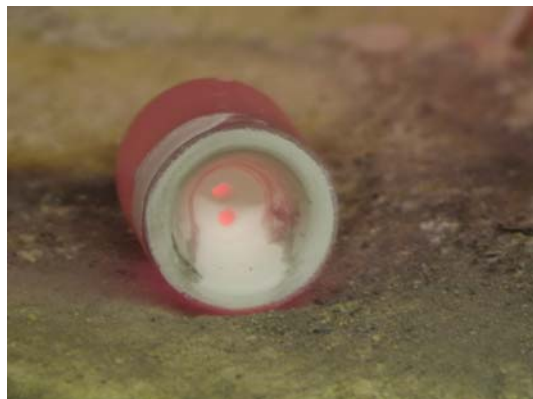
(32) Red-hot casting ring after wax burn out
