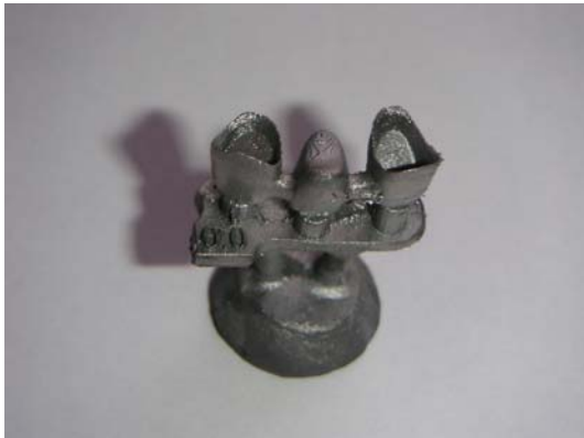
(37) Later photopolymer cast after matching investment expansion coefficients
