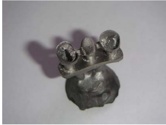
(36) Early cast showing flashing due to photopolymer expansion investment cracking
