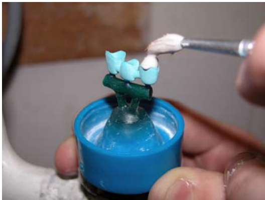
(29) Applying investment by hand to delicate areas before investing
