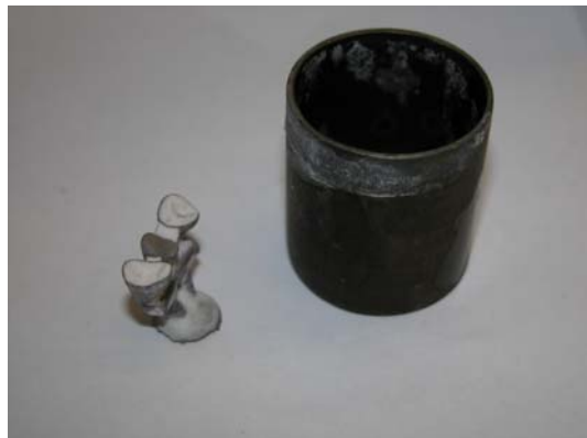
(33) Induction melting alloy and centrifugal casting
