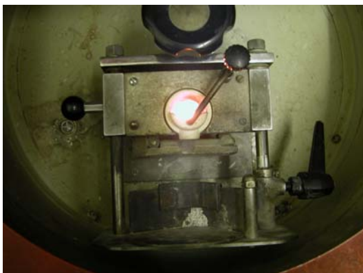
(33) Induction melting alloy and centrifugal casting
