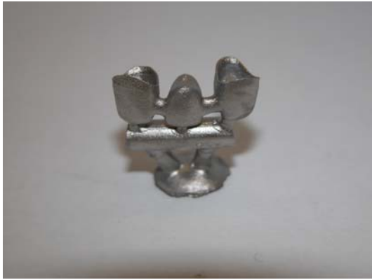
(35) Casting after sandblasting and glass beading
