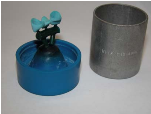
(27) Wax pattern, reservoir and sprue ready for investing
