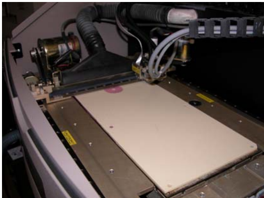
(21) Manufacture Method #3: 3-D wax jet printing
