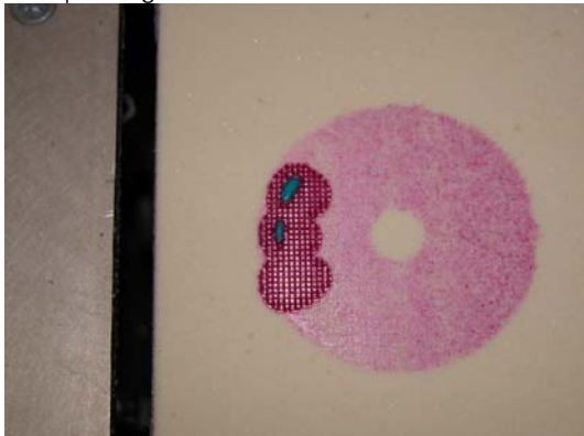
(23) Detail showing wax support structure build
