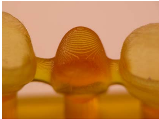
(20) 3-unit photopolymer bridge framework detail
