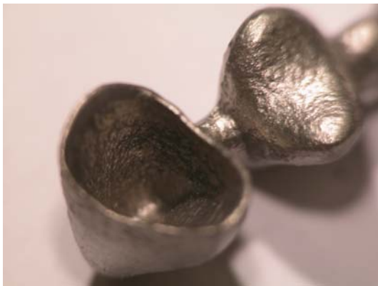
(39) Casting from wax jet model – note improved quality due to wax burn out
