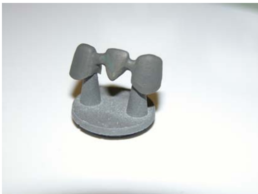
(41) Casting after oxidation
