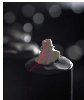
(3) Laser Scan of Plaster Cast from patient impression (accuracy ~15 micron)
