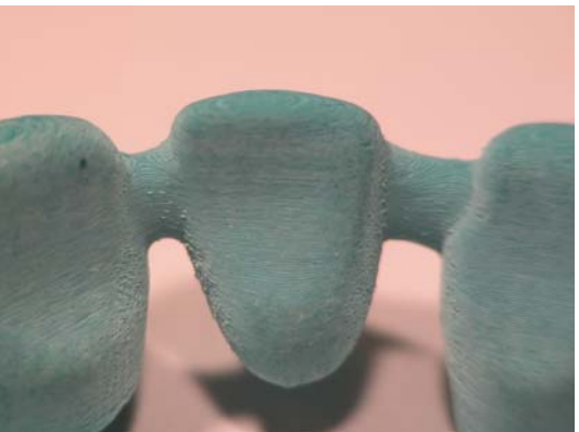
(26) 3-unit wax bridge framework detail (note improved resolution over photopolymer)
